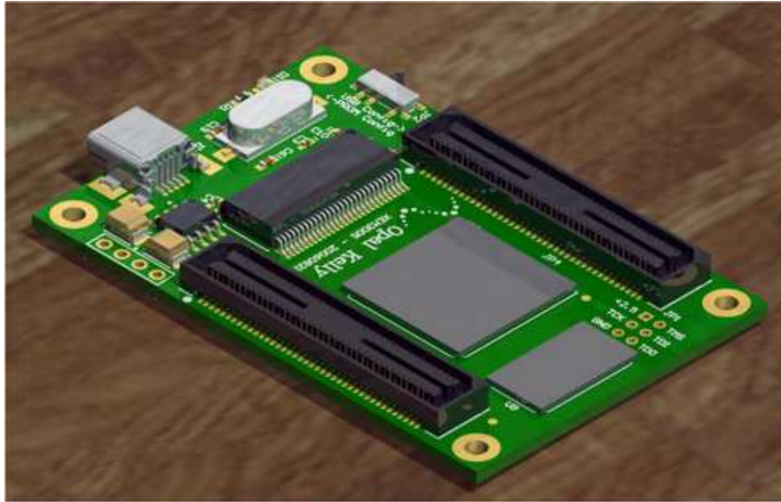
Figure 12 : Opal Kelly XEM3005 FPGA Board. Model provided by Opal Kelly and rendered in Solidworks Photoworks.
