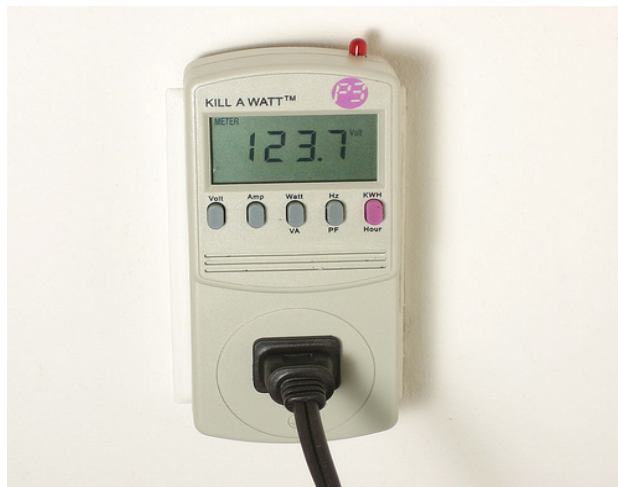
Figure 1. Kill-a-Watt modified into a Tweet-a-Watt. The LED at the top flashes each time the Tweet-a-Watt transmits a data packet.
