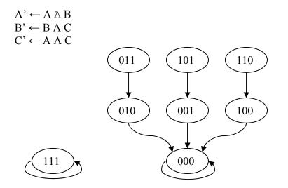
Figure 2. An example of a 3-gene network with two attractors
