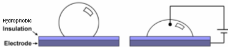
Figure 2: Electrowetting. The application of a voltage to the droplet creates a charge at the liquid/insulator interface, resulting in a wetting force at the contact line that changes the contact angle of the droplet.
